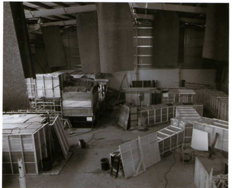
The tunnel sets
